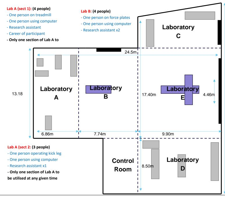
Equipment locations within the lab, some items are immovable due to the weight of the machine (i.e. >150kg)
